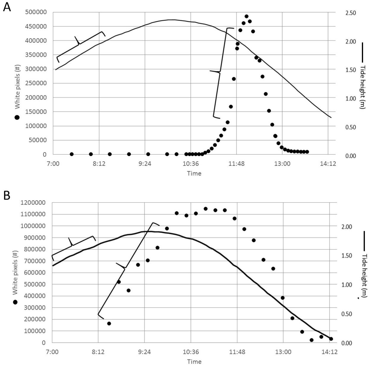
**FIGURE 3. Estimated marsh inundation and tide-based change in sea elevation for one tide cycle. Change in reflected light (# white pixels) and sea elevation (tide) for: (A) a mid-high tidal, pickleweed-dominated marsh and B) a mid-tidal, bulrush-dominated marsh. Brackets indicate the range of tide heights and marsh area used to calculate rate of water elevation change and rate of inundation.**
