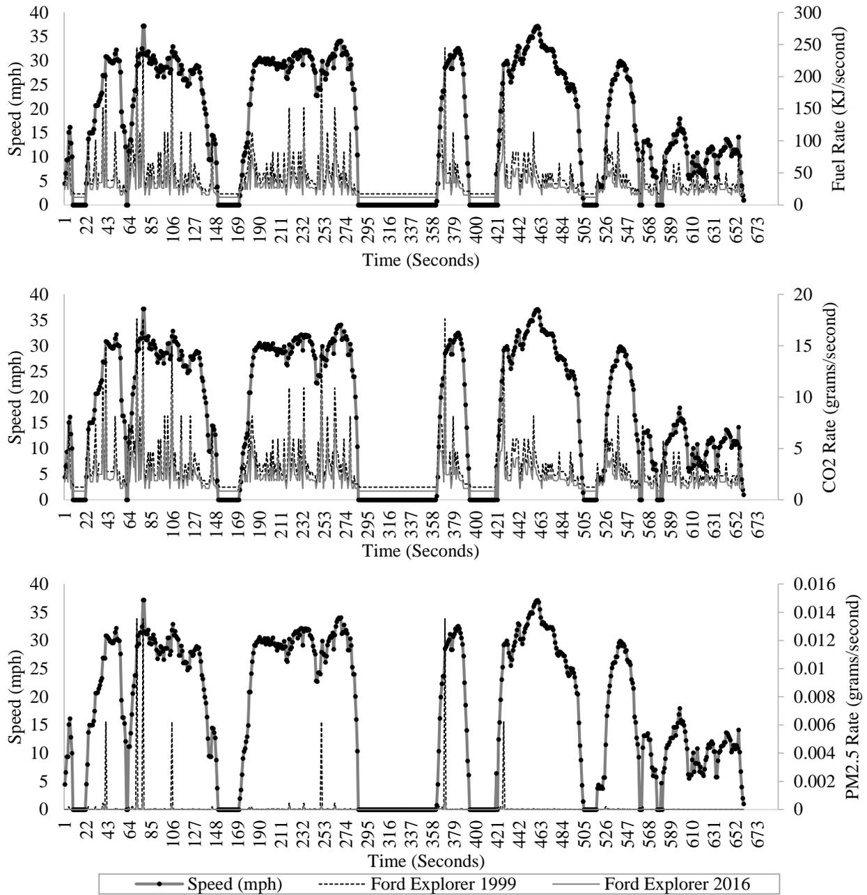
**FIGURE 5 Second-by-Second Speed, Fuel Consumption and Emission Rate\***
