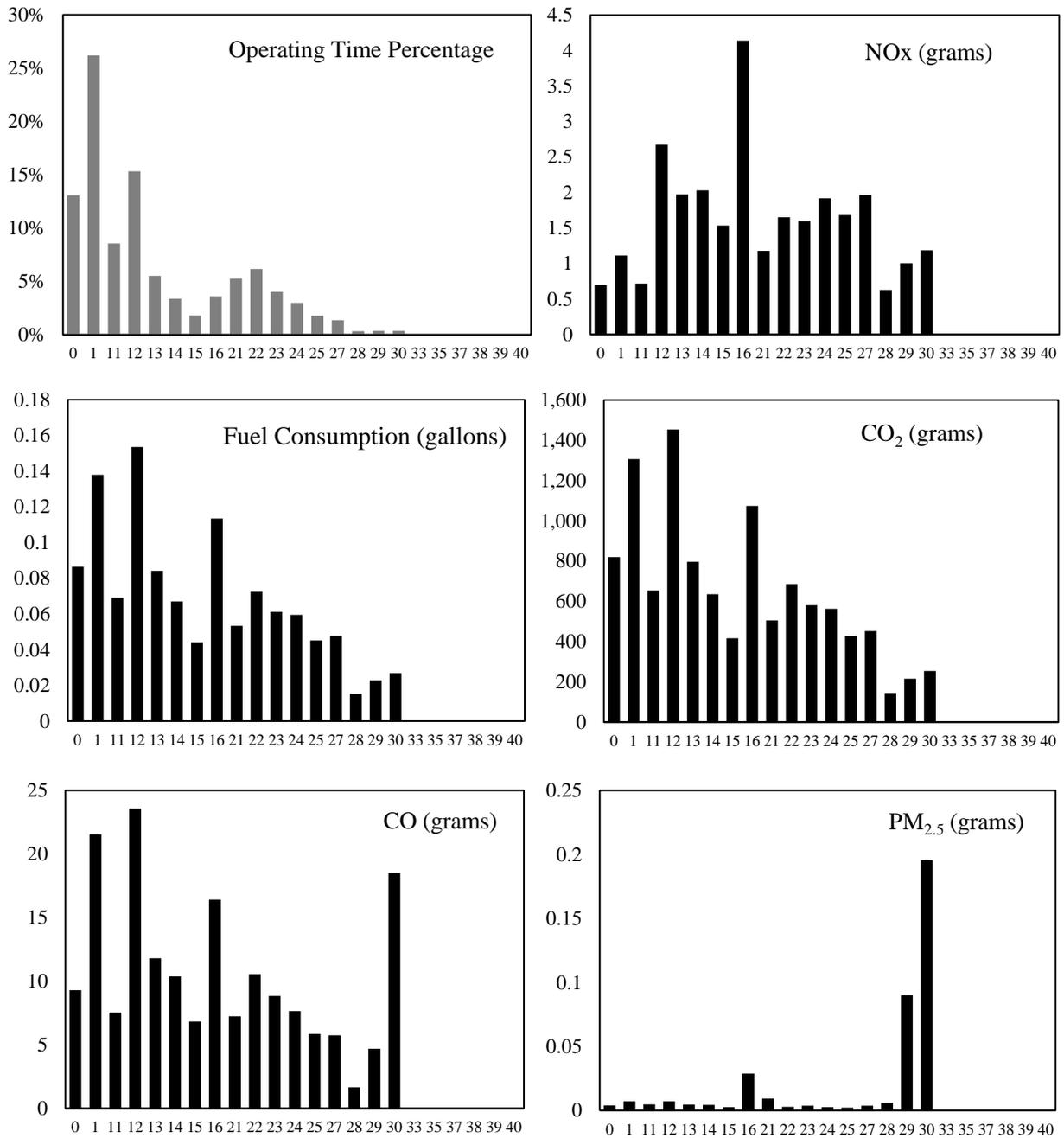
**FIGURE 6 Operating Time Percentage and Emissions for Each Operating Mode Bin for the 1999 Ford Explorer\***
