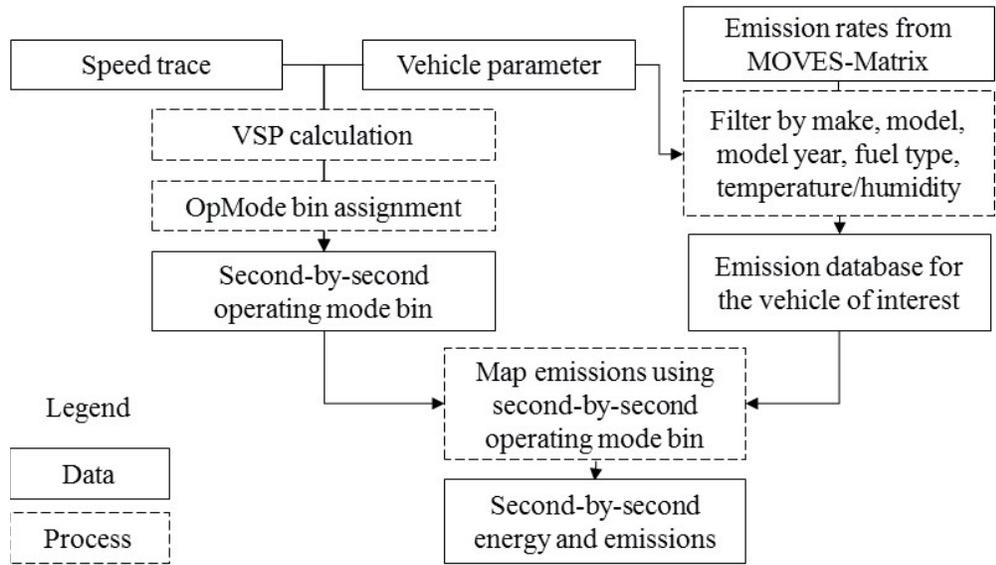
**FIGURE 2 MMC Algorithm Design**
