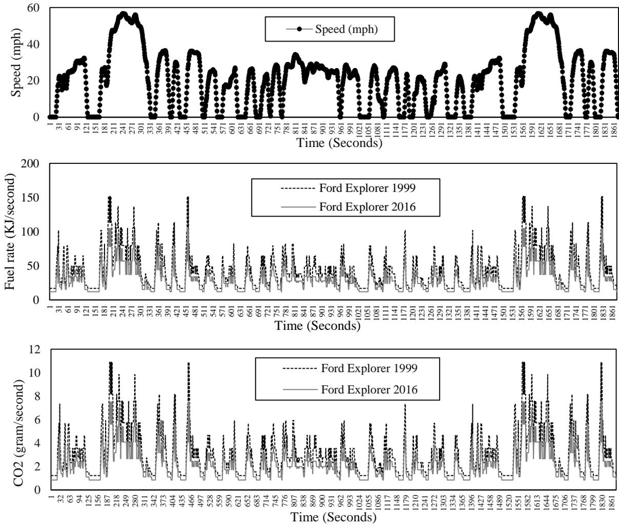
**FIGURE 3 a) FTP/EPA75 Second-by-Second Driving Cycle, b) Fuel Consumption Rate, and c) CO2 Emission Rate\***
