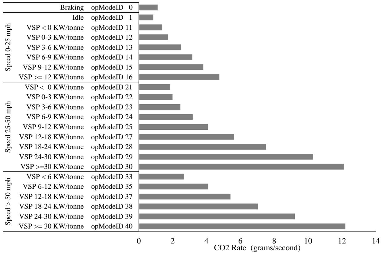
**FIGURE 1 Example CO2 Emission Rates by VSP Bin for Passenger Trucks (MY 2016)**
